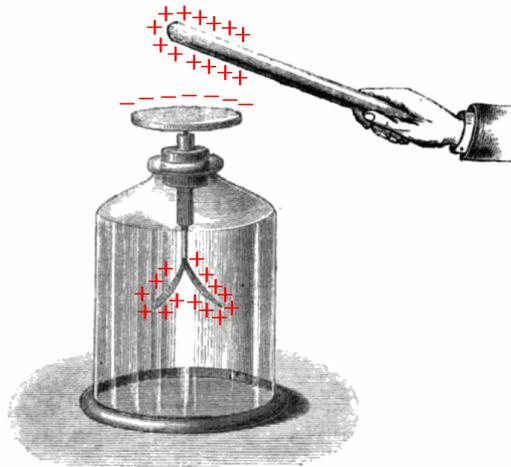
Figure 6.1: Electroscope charged by induction. Source: Sylvanus P. Thompson (1881) Elementary Lessons in Electricity and Magnetism, MacMillan, New York, p.16, fig. 12
